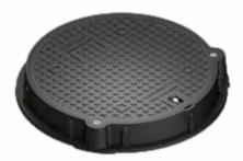
SMC composite manhole cover D 400 with extractible hinge and vents clear opening 600 with two screws
